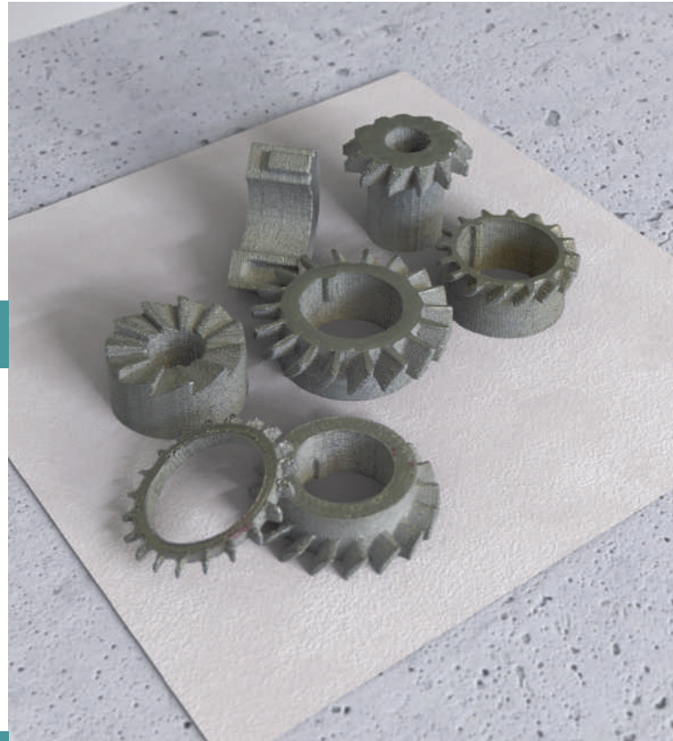
AIM3D 3D printing technology provides a wide range of material options, including various grades of stainless steel, aluminum, titanium, and Inconel.
